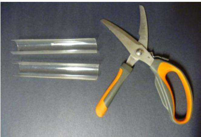
Use shears or scissors to cut plastic or cardboard tubing in half lengthwise to create basic ramps.
