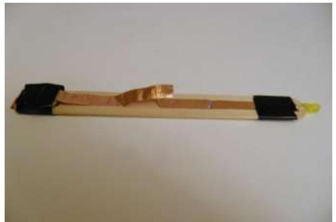
Attach the LED light to the other end of the popsicle stick. Make sure the LED leads are in contact with the copper tape.
