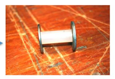
Slide a washer onto each end of the gluestick.
