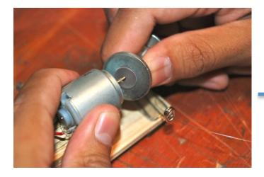
Push the center of the gluestick onto the motor.
