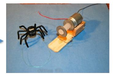
Connect the electrical wires to a battery. Put a momentary switch in the system if you have one – if not, you can always manually connect and dissconnect the wire to the battery. Hang the spider over the edge of a table and turn on the motor to watch it crawl upwards!
