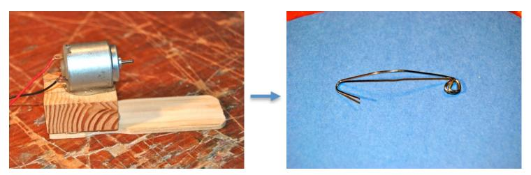
Build a base using a paint paddle and small block of wood. Glue the motor onto the base.
