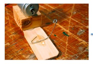
Glue the paperclip onto the base as shown. Wait for glue to cool and dry.
