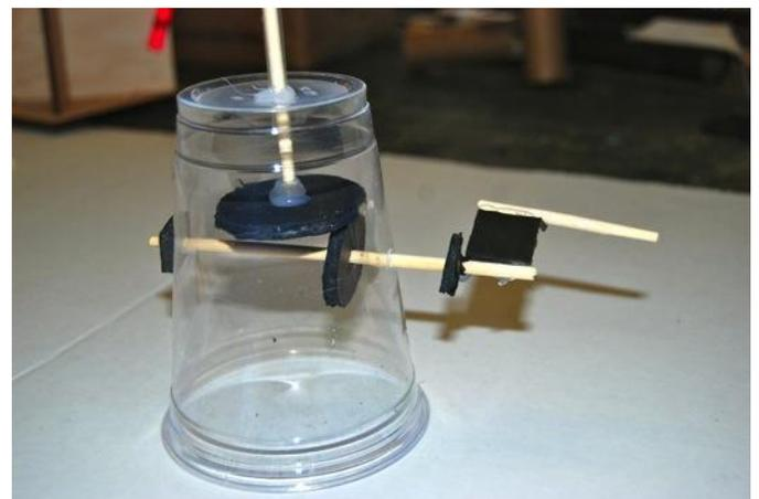
Glue the handle to the crankshaft. You have just created a crank!
